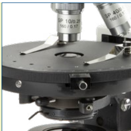
360° rotatable circular stage for polarization
